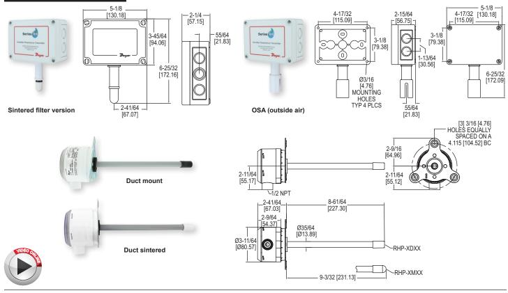
The Series RHP Temperature and Humidity Transmitters combine the voltage or current humidity transmitter output with a passive temperature thermistor or RTD output. Featuring polymer capacitance humidity sensors, models are available with 2%, 3% or 5% accuracies. Duct mounted transmitters are available with an optional two-line alpha numeric LCD display.
