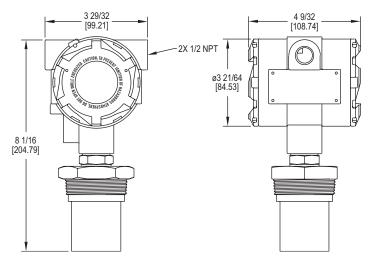
The **Series ULT Ultrasonic Level Transmitter** provides non-contact measurement of liquid levels in an explosion-proof body. It is capable of measuring up to 32.8' (10 m) with a PVDF sensor and 4-20 mA output.
