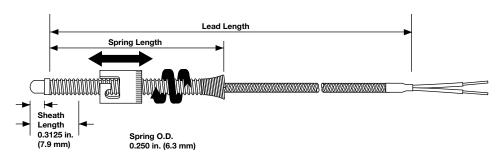
Adjustable spring style thermocouples bend to any angle to fit a wide range of hole depths, eliminating the need to stock numerous styles.
