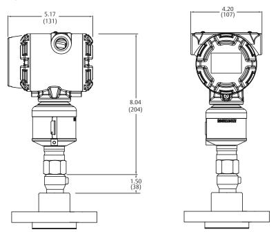
Lower housing (flushing ring) is available with FFW style flange.
