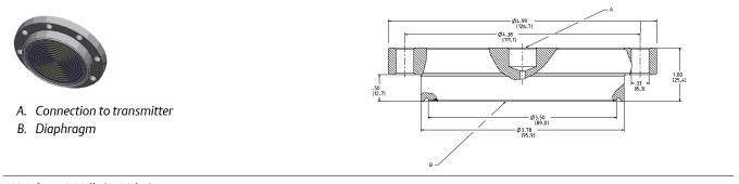
Weight = 4.18 lb (1,88 kg) Dimensions are in inches (millimeters).
