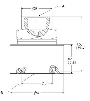
Weight = 1.33 lb (0,60 kg) Dimensions are in inches (millimeters).
