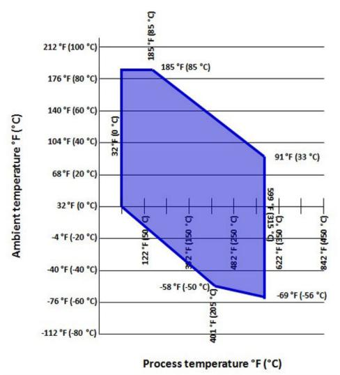
Figure 13: Thermal Optimizer with Silicone 704 Fill Fluid Temperature Limits
