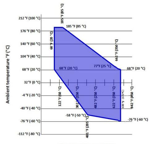
Figure 14: Thermal Optimizer with Silicone 705 Fill Fluid Temperature Limits
