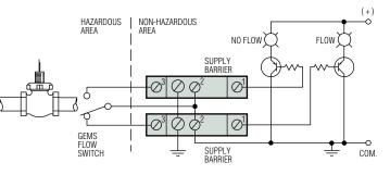
Used with GEMS flow switch located in a hazardous area for flow/ no flow indication.
