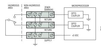
For optically coupled microprocessor. 65800 Series supply with two return barriers for SPDT switch.
