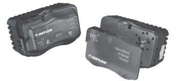
The SERIES EHG<sup>®</sup> is an integrated multi-function controller that is a key component in a powerful system that integrates a heater, an adjustable set point temperature controller, a high/low temperature alert, a power switching device and a high temperature safety limit. The agency recognized controller/safety limit meets UL<sup>®</sup> and CE requirements.
